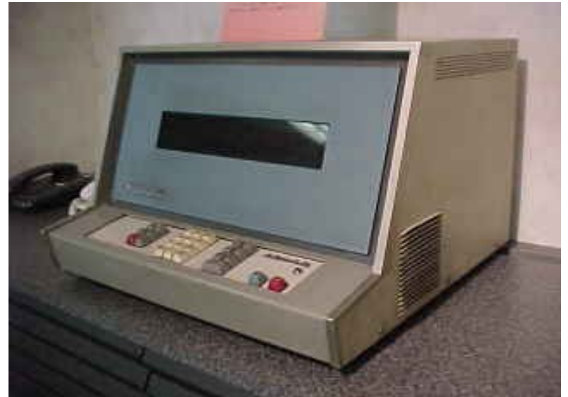
Oi Electric Parametron X-8-01, 1964 Ferro-Electronic Calculator
